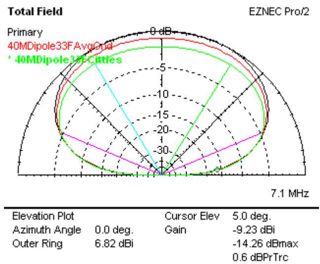
Fig 24 - The Effect of Ground on a 40M Dipole at 33 Ft
