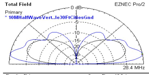
Fig 15 - 10M  $\lambda/2$  Dipole at 6 in, 33 Ft Very Poor (Cities) Ground
