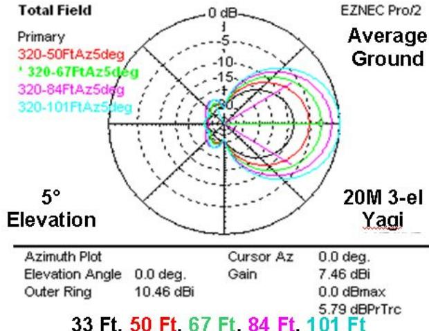
Fig 38 – 20M Yagi vs Mounting Height
