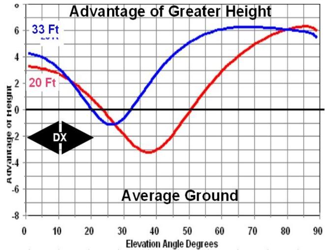
Fig 3 - Loaded 20M Dipole at 20 Ft, 33 Ft compared to same antenna at 3 ft
