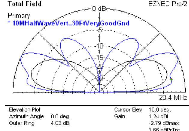
Fig 17 - 10M  $\lambda/2$  Dipole at 6 in, 33 Ft
