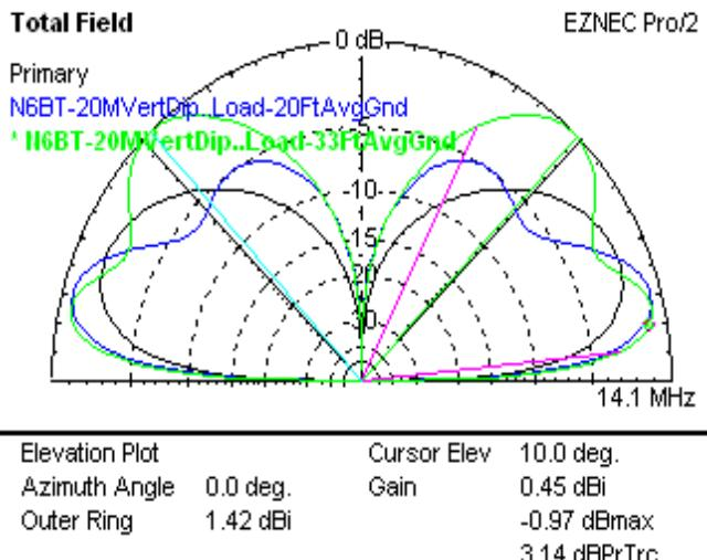
Fig 2 - Loaded 20M Dipole, 3 Ft, 20 Ft, 33 Ft Average Ground
