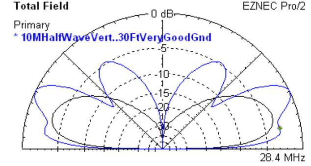
Fig 17 - 10M  $\lambda/2$  Dipole at 6 in, 33 Ft Very Good Ground
