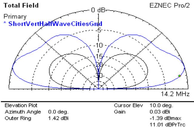
Fig 22 - Very Short 20M Dipole at 6-in, and 33 Ft, Very Poor Soil
