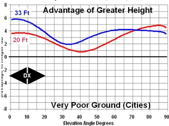
Fig 6 - Loaded 20M Dipole, at 20 Ft, 33 Ft
