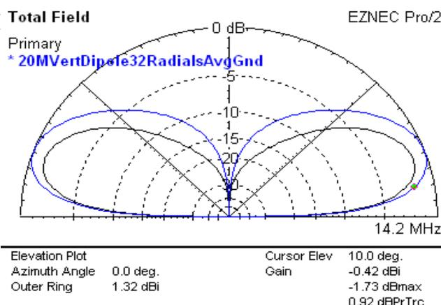
Fig 19 - Radials for a Half Wave Dipole Average Ground
