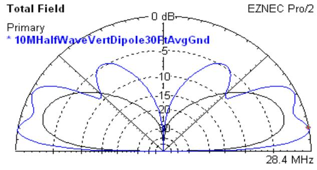
Fig 16 - 10M  $\lambda/2$  Dipole at 6 in, 33 Ft Average Ground
