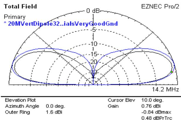
Fig 20 - Radials for a Half Wave Dipole Very Good Ground
