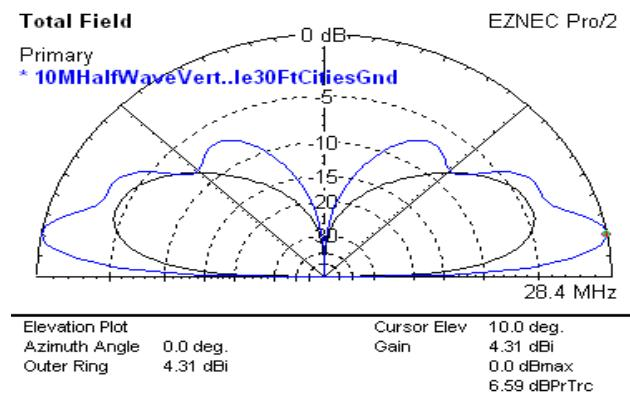
Fig 15 - 10M  $\lambda/2$  Dipole at 6 in, 33 Ft
