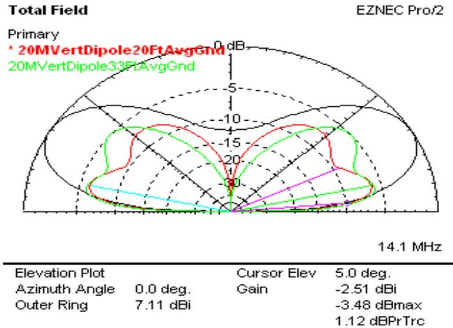
Fig 30 - 20M Horizontal Dipole at 33 Ft,  $\lambda/2$  Vertical Dipole at 20 Ft and 33 Ft Average Ground
