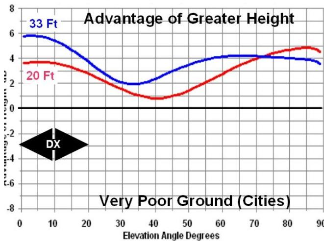
Fig 6 - Loaded 20M Dipole, at 20 Ft, 33 Ft compared to same antenna at 3 ft
