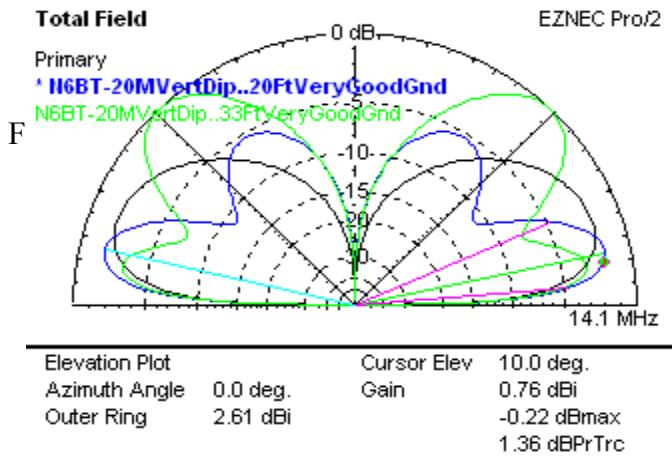
Fig 5 - Loaded 20M Dipole, 3 Ft, 20 Ft, 33 Ft
