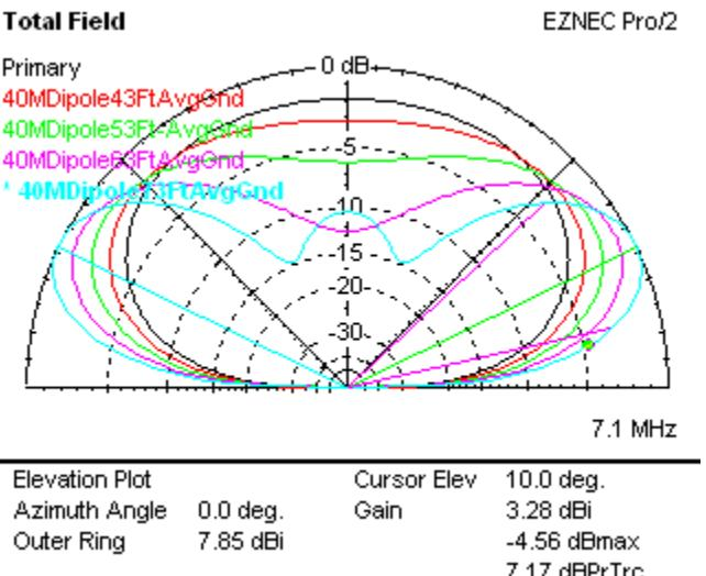
Fig 25- The Effect of Height on a 40M Dipole over Average Ground
