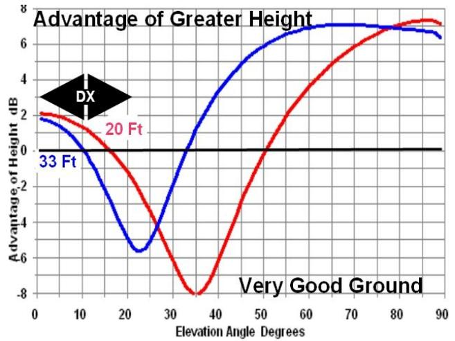
Fig 7 - Loaded 20M Dipole, 3 Ft, 20 Ft, 33 Ft compared to same antenna at 3 ft
