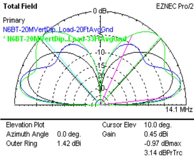
Fig 2 - Loaded 20M Dipole, 3 Ft, 20 Ft, 33 Ft Average Ground
