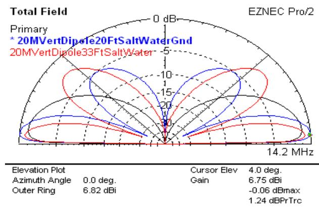
Fig 21 - 20M Vertical Dipole at 20 Ft and 33 Ft Over Sea Water
