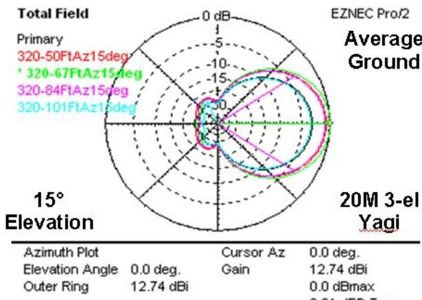
Fig 40 – 20M Yagi vs Mounting Height
