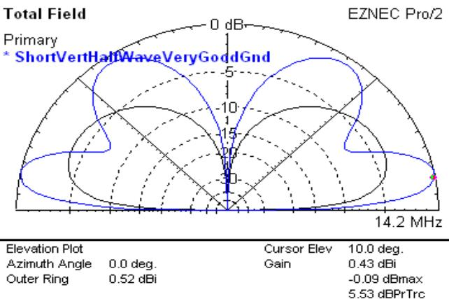
Fig 23 - Very Short 20M Dipole at 6-in, and 33 Ft, Very Good Soil
