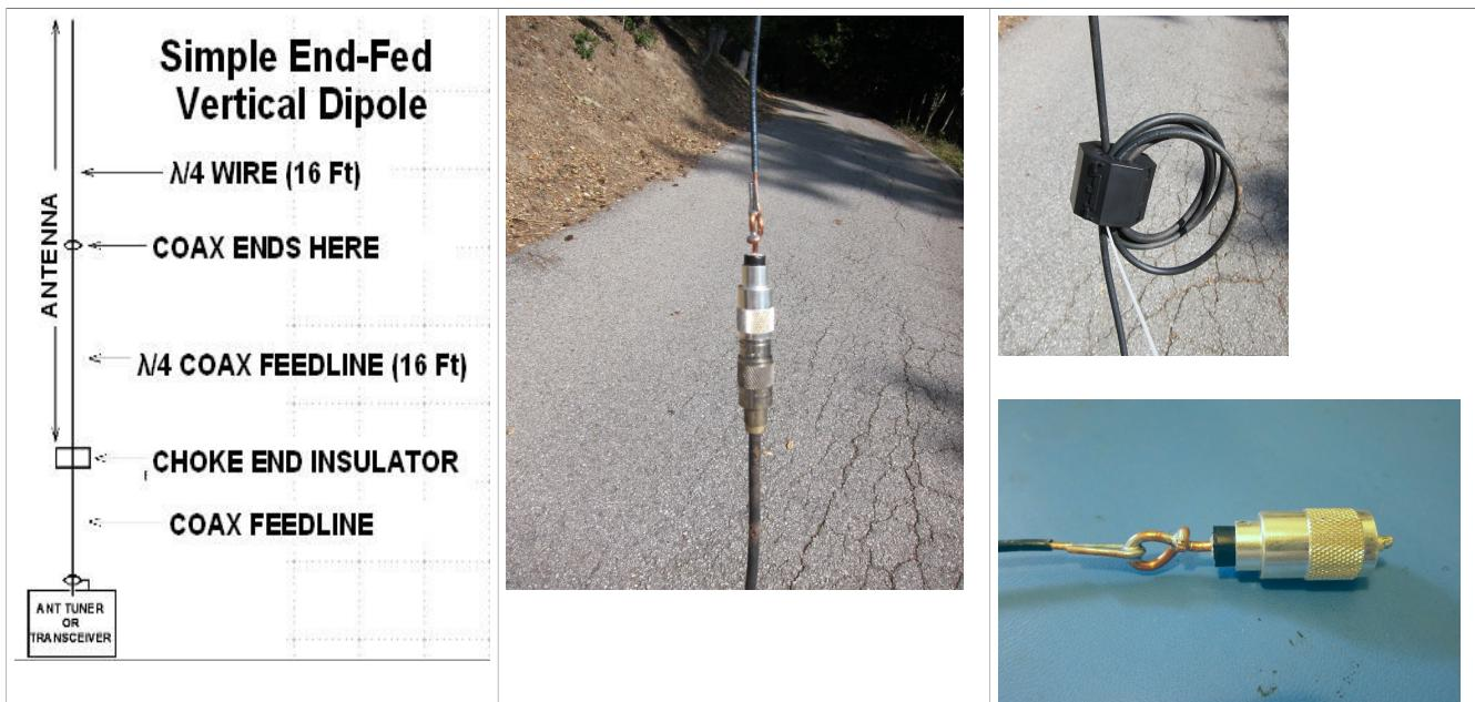
Signal strength measurements were made with the dipole center at ground level and the feedline laying on the ground to form a quarter-wave vertical with a single radial; then with the choke 6-inches above ground level, forming a half-wave dipole with its base 6-inches ground level; then with the dipole raised in 10 ft increments to a maximum height of 40 ft above ground. My RX antenna was a 20M vertical with two radials laying on the ground. Results are shown below.
