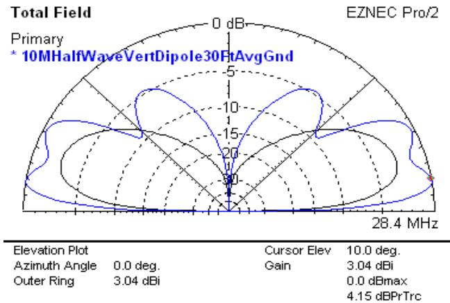
Fig 16 - 10M  $\lambda/2$  Dipole at 6 in, 33 Ft
