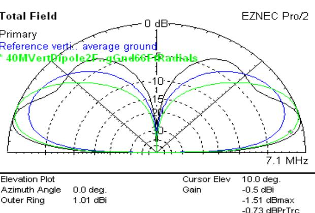
Fig 11 - Ground-mounted  $\lambda/4$ ,  $\lambda/2$ , and  $5\lambda/8$  tall
