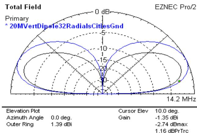
Fig 18 - Radials for a Half Wave Dipole Very Poor Ground
