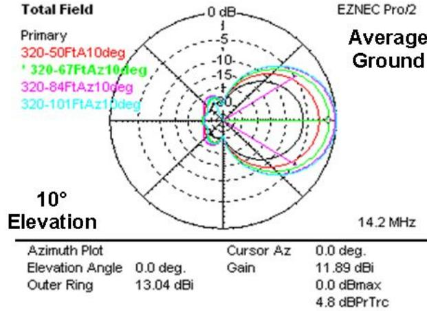
Fig 39 – 20M Yagi vs Mounting Height
