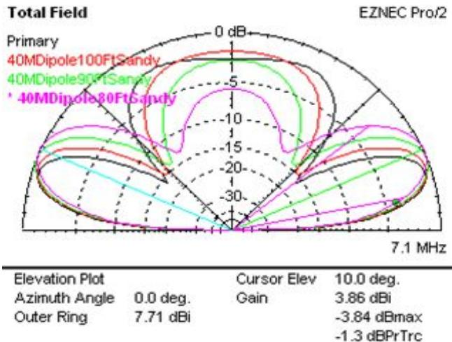
Fig 32 - 40M Horizontal Dipole at 80 Ft, 90 Ft,
