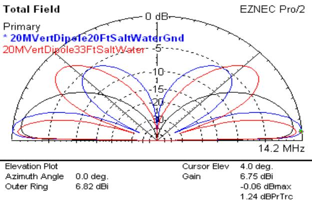
Fig 21 - 20M Vertical Dipole at 20 Ft and 33 Ft
