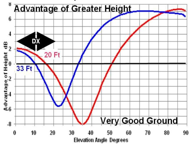
Fig 7 - Loaded 20M Dipole, 3 Ft, 20 Ft, 33 Ft
