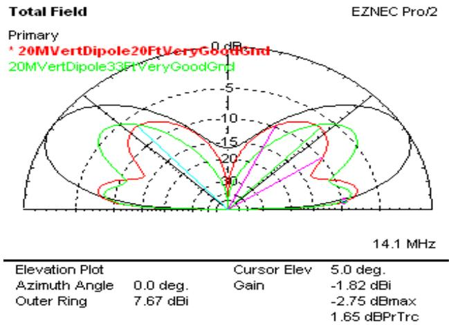
Fig 31 - 20M Horizontal Dipole at 33 Ft,  $\lambda/2$  Vertical Dipole at 20 Ft and 33 Ft. Very Good Ground
