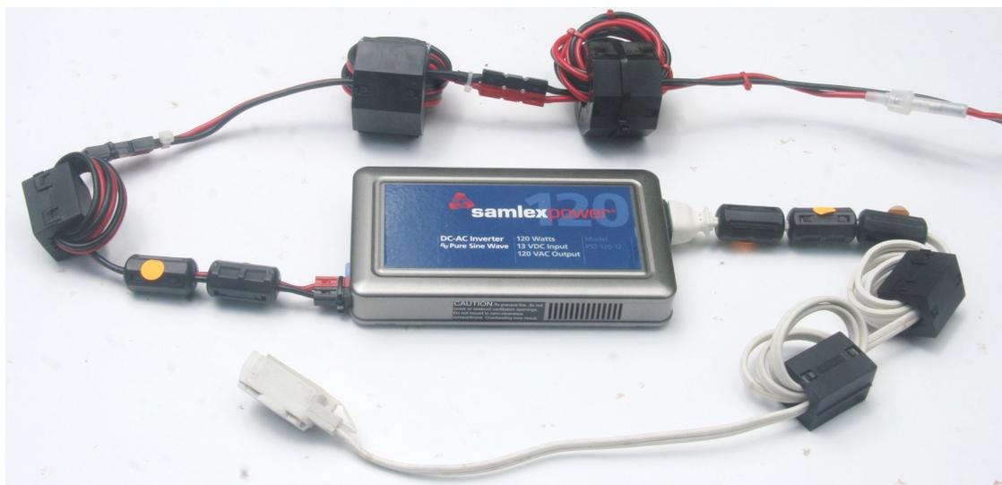
Fig 11 – 12VDC to 120VAC 1A Inverter with Required RF Filtering
