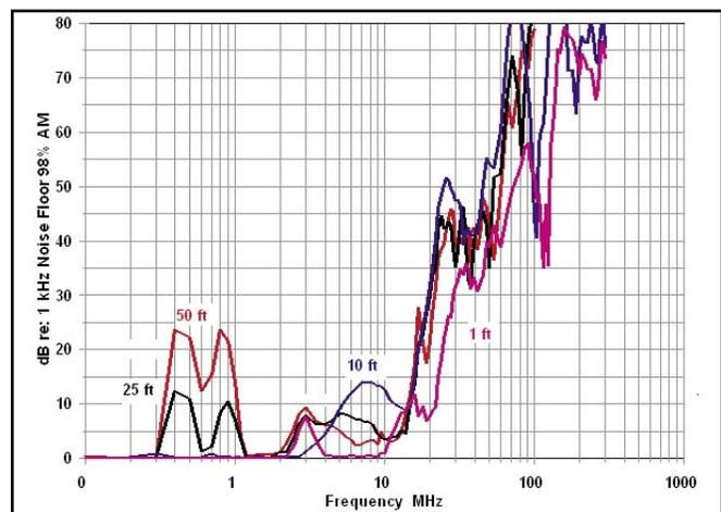
Fig. 5 – A mic with severe susceptibility to VHF RF.
