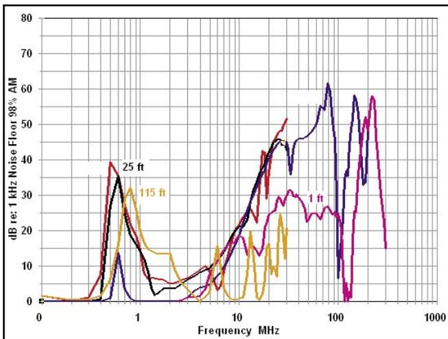
Fig 8 -- This mic had no problem with the AM broadcast transmitter, but it did receive interference from the ham transmitters and from some VHF TV.
