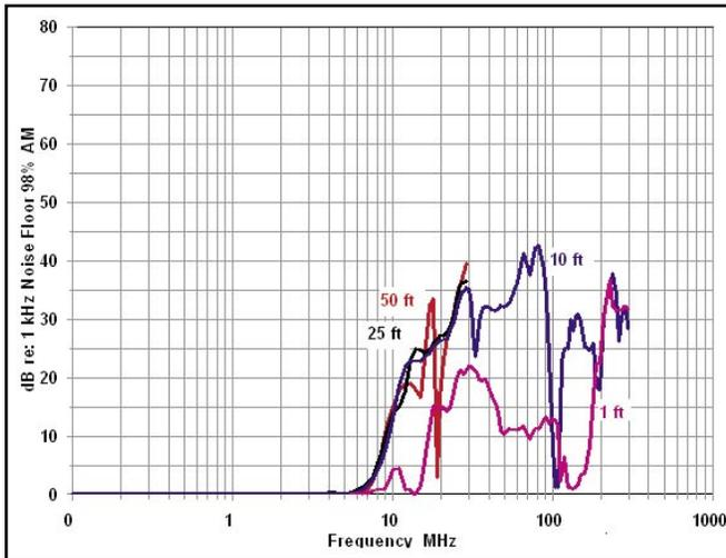
Fig. 6 – This mic experienced moderate interference from the ham transmitters in the 10-30 MHz range.
