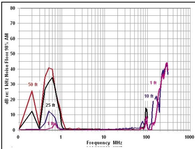
Fig. 7 – This mic has sufficient filtering to reject all but the strongest RF below 200 MHz. It experienced no interference from the AM broadcast or ham transmitters.
